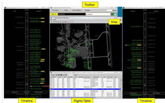
Figure 2. STBO Client – main interface for ATCT TMC.
